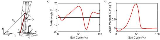
Figure 1 – a) Representation of a generic rigid body using the FCC-GRB Formulation with one MTU; b) Ankle joint angular displacement during gait; c) Moment of force at the ankle joint during gait.
